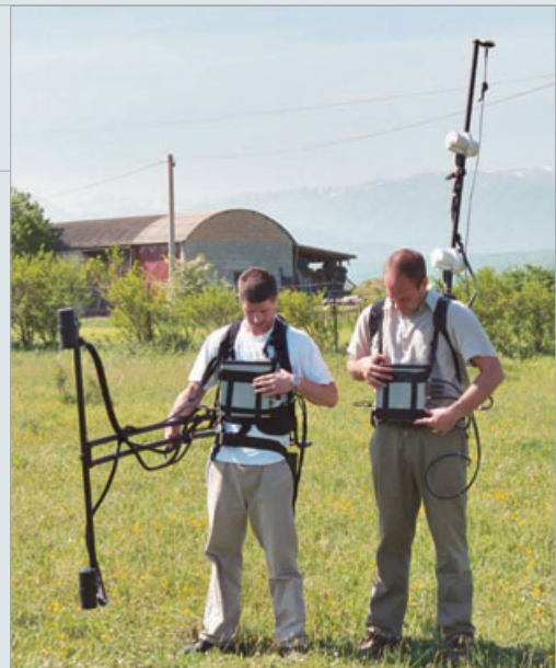
OSI equipment demonstration, Italy: magnetometers.
