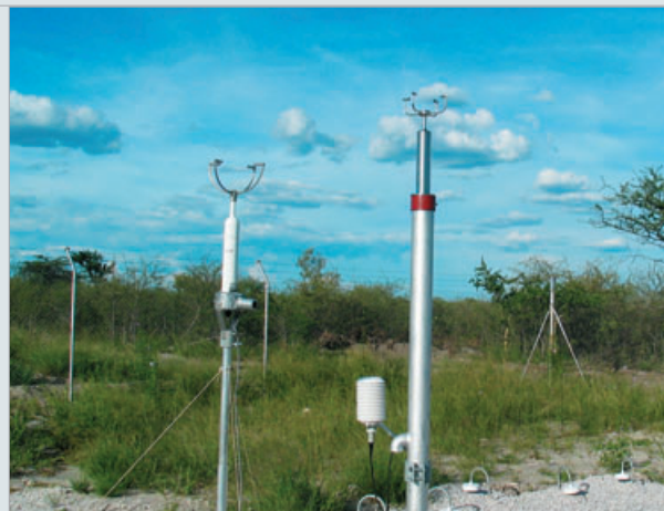
Equipment set-up for checking meteorological data during certification visit at infrasound station IS35, Tsumeb, Namibia.
