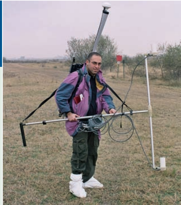
High resolution geomagnetic survey during the OSI advanced training course in Szolnok, Hungary.
